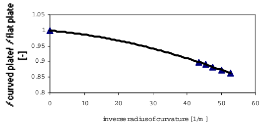
Figure 2. Graphical presentation of the ratio of resonant frequencies against the inverse radius
